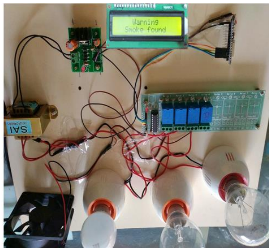
Figure 4. Hardware output when spoke will be detected
