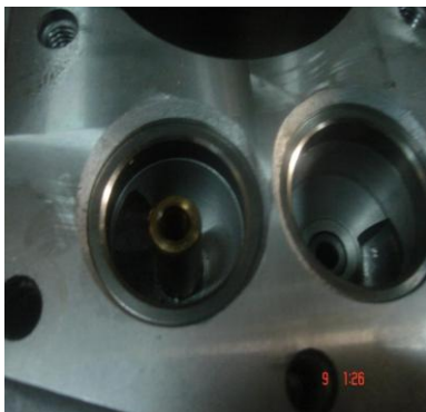
Figure 5, shows a valve pulled in position.
