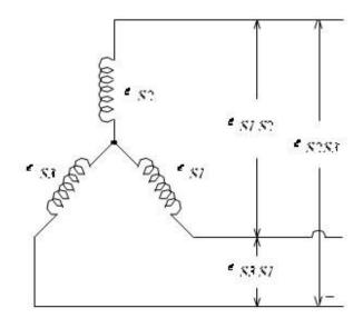
Fig.2 Induced emf in stator coils
