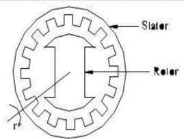
Figure.1 Constructional Features of Synchronous Transmitter
