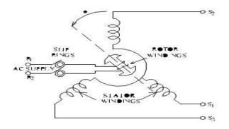
Figure – 3 Electrical Circuit (Synchronous Transmitter )
