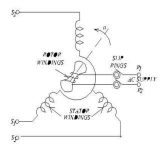
Fig.1 Electrical Circuit of synchronous control transformer
